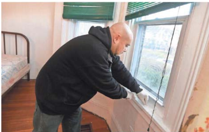
City of Rochester inspector Ricardo Nieves swabs a windowsill of an apartment as part of a lead-screening process.
